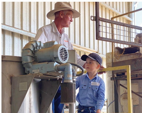
Aeromaster TE-500 Tea Extraction Unit produces extracted Liquid Humus Tea for foliar, fertigation or liquid injection.
